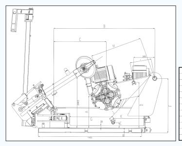
This 3-phase machine is capable of changing tyres on rims from 14" (355mm) to an impressive 46" (1168mm) in standard configuration but the addition of extensions increase this to a huge 56" (1422mm). Tyres up to 103" (2600mm) in diameter and 59" (1500mm) wide are handled with ease. The industrial strength gearbox and clamping chuck allow the megamount 852 to operate in the harshest conditions, such as mining facilities and military field operations.
