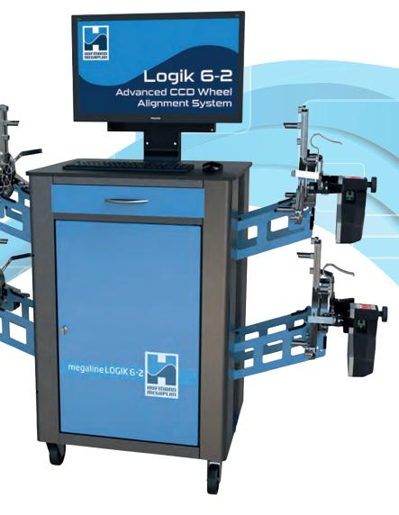
The Logik 6-2 can also be used on a 2 post or mid-rise scissor lift using the optional kit.
